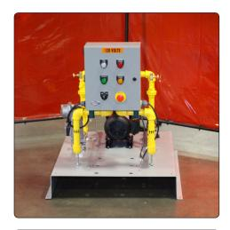
The E101-P is designed as a Plug and Play unit and comes completely prepiped, wired and tested for your application with: Metal skid-style frame with all components mounted and wired. · UL /CSA approved gas booster pump and components. • 1/3 HP TEFC motor, 120/1/60. • 1" NPT union ends inlet and outlet for easy installation.
